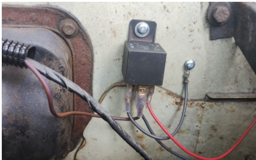
A 12V relay and inline fuse are ideal for running the fuel pump
