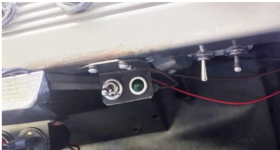
The switch and warning light are positioned discreetly below the dash.
